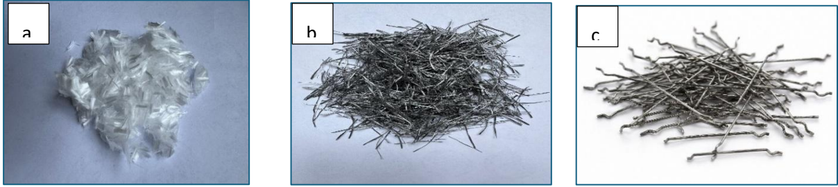
Görsel 1. A) Polipropilen Lif – b) Macromesh Lif – c) Çelik Lif
