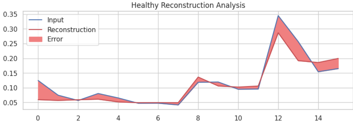
Figure 3. Healthy reconstruction analysis based on the autoencoder output.
